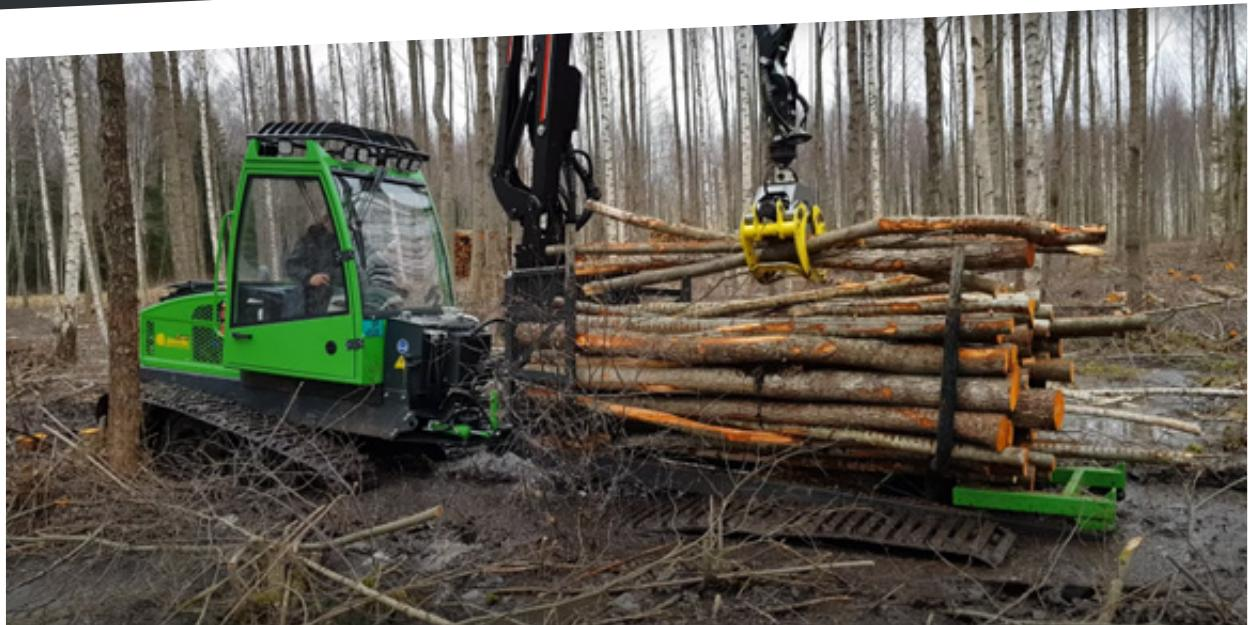
Thanks to the minimal ground pressure, low centre of gravity and high ground clearance, the machines are capable of operating in difficult conditions, such as crossing deep ditches.
